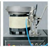
Elevate your Hardware Insertion Press with our Brush Table attachment. Designed to minimize friction and static, this addition ensures optimal efficiency, reducing the risk of damage and cosmetic imperfections caused by repositioning the part prior to inserting hardware.
