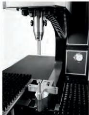
The Sanson offers a quick change auto feed system for standard nuts, studs and standoffs. Top feed and bottom feed tooling allow for maximizing productivity and minimizing downtime.
